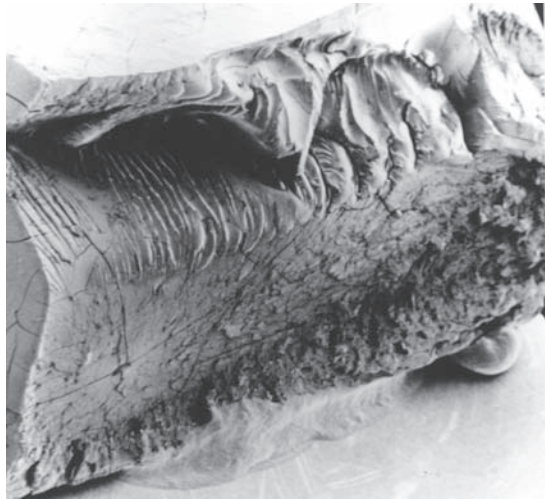
Fig. 8.3 (a) and (b) Failure in samples of starch/glycerol (80:20 weight/weight of non-aqueous components); water content of sample is (a) 6.5% (wet weight basis) and (b) 9.9% (wet weight basis) (from Kirby et al. , 1993). (c) and (d) Failure in cooked meat (from Purslow, 1985).
